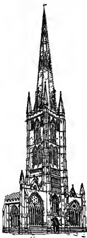
C ST WULFRAN GRANTHAM, LINCS. PARAPET ANGLE TURRETS & CROCKETS
